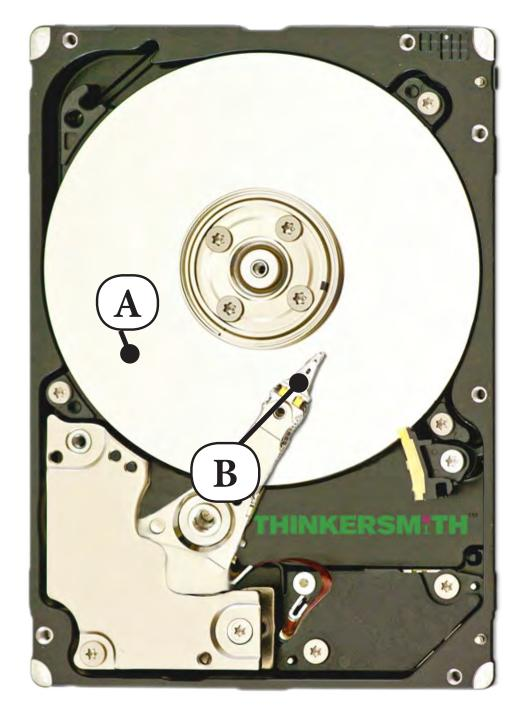
A) Spinning Storage Platter B) Read/Write Head
