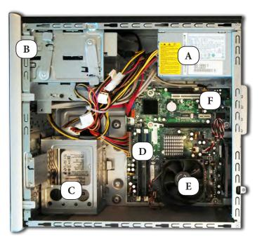
Do you see that big silver box with all of the wires under the label A? That's the **Power Supply**. It converts the power that comes from the wall outlet into something that the computer can use. It then feeds that power to the rest of the computer parts.
