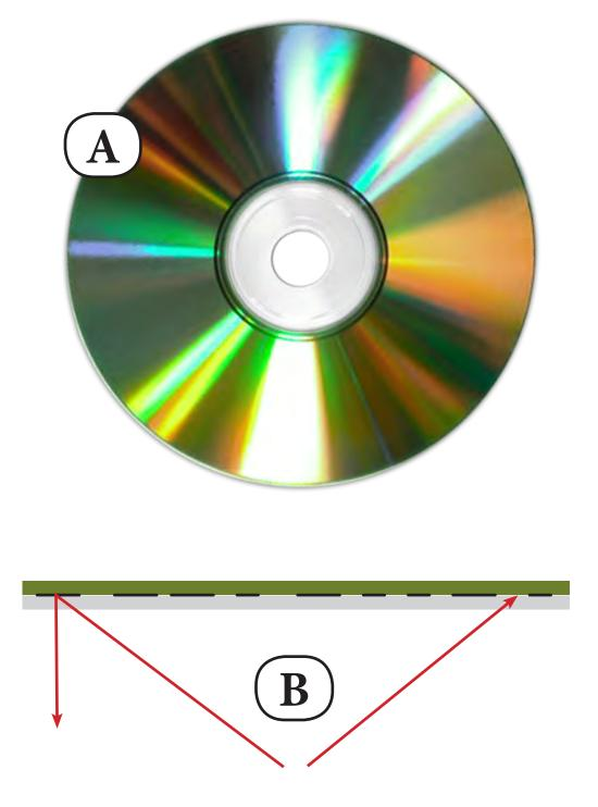
A) Front View B) Side View with Laser Direction
