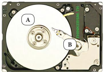
A) Spinning Storage Platter B) Read/Write Head
